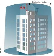
The protection level is set according to numerous parameters including loss of life and economic risks, the average local lightning striking, the impact on environment, etc... To favour an ideal matching to the layout of the different premises to protect, Paraton@ir® is available with 4 power levels.
